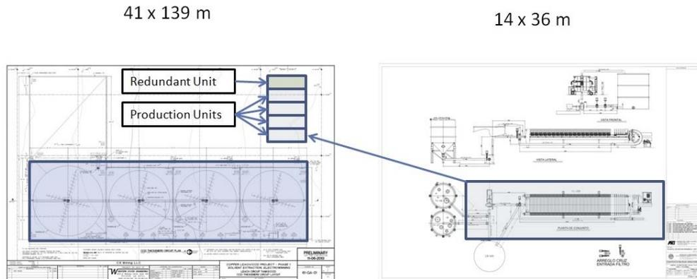
Clearly, one can see that the AFT footprint reduces the processing area footprint by about 85%.
